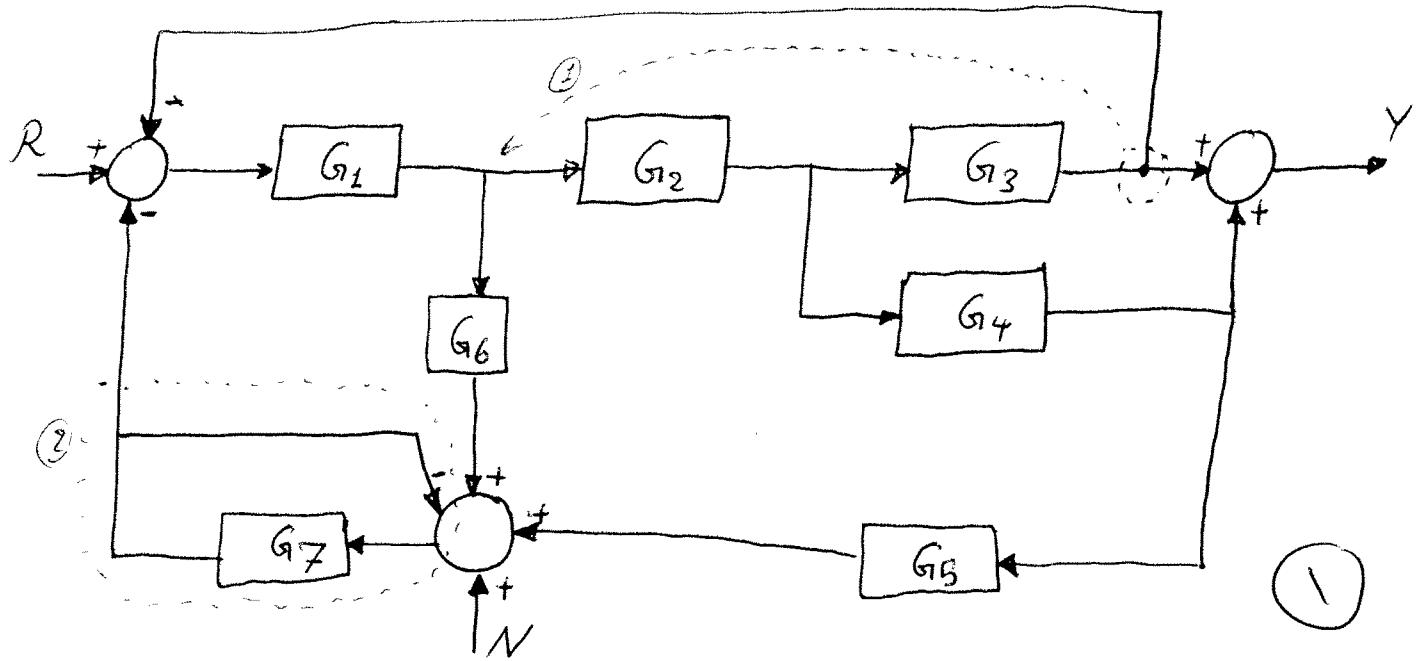
① Moving the take-off-point (from output of  $G_3$  to input of  $G_2$ )
