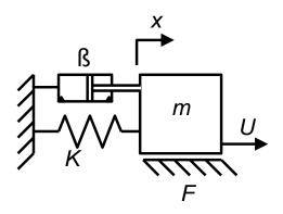
2. Derive the differential equations that represent the mechanical system shown, where U is a force that affects the mass  $M_1$  and hence derive the transfer functions  $X_1(s)/U(s)$  and  $X_2(s)/U(s)$ . If the force U has a value of 1 N find the steady state values of  $X_1$  and  $X_2$ .
