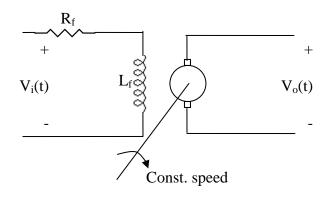
5. The system shown in the figure consists of a DC- generator connected to RC impedance. Find the differential equation and the T.F that relates  $V_i$  and  $I_o$ .
