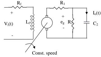
6. A schematic diagram of a generator-motor system driving an inertia load J with viscous damping B at an angular velocity  $\theta$  is shown in the figure. Given that the torque constant of the motor and its induced back emf constants are  $K_T$  and  $K_m$  respectively and the generator constant is  $K_g$ . Derive a mathematical model for determining the motor output speed and hence find the transfer function of the system.
