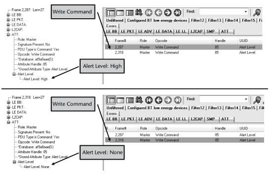
Figure 15.15 Read or write alert level characteristic.
