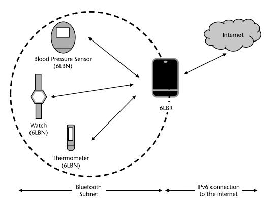
Figure 15.9 Typical configuration of a BLE network connected to the Internet.
