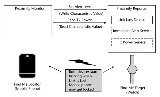
Figure 15.4 Immediate alert service, link loss service, Tx power service, and proximity profile roles.
