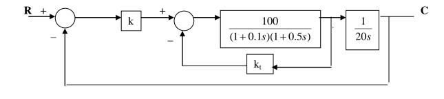
4. The block diagram of a feedback control system is shown in the figure. The error signal is defined to be e (t).
