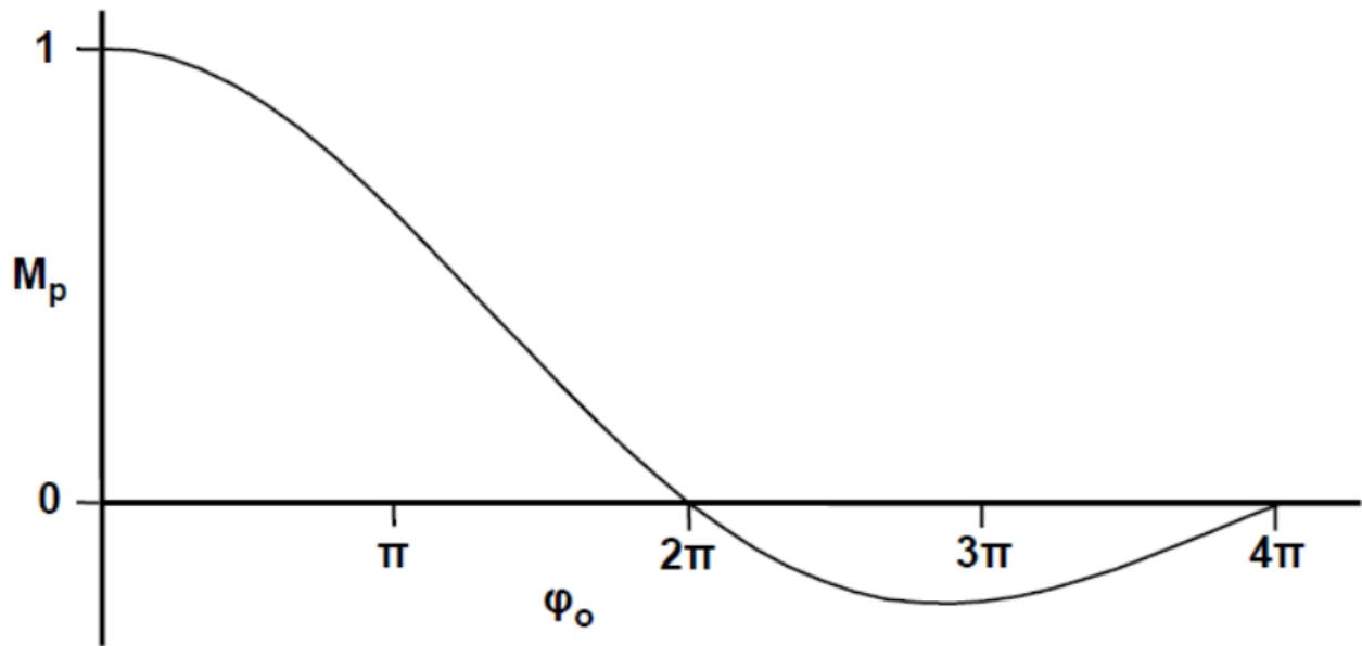
$$M_p = \frac{\sin(\varphi_0/2)}{\varphi_0/2}, \quad \varphi_0 = \omega T = \frac{\omega \ell}{u_0}$$
