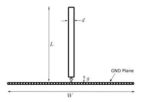
The parameters shown in the figure are: monopole length  $L=35.625\,\mathrm{mm}$ , square ground plane width  $W=200\,\mathrm{mm}$ , wire diameter  $d=0.3\,\mathrm{mm}$ , and gap width where discrete port excitation is placed g=L/200.
