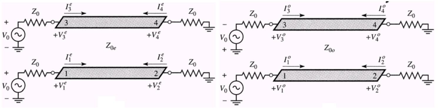
$$V_1^e = V_0 \frac{Z_{in}^e}{Z_{in}^e + Z_0}, \quad V_1^o = V_0 \frac{Z_{in}^o}{Z_{in}^o + Z_0}$$
