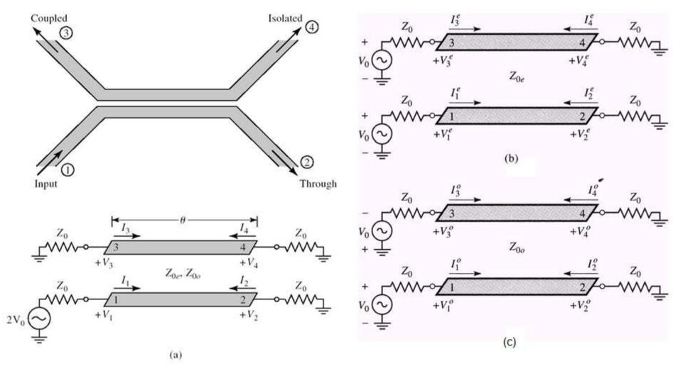
Circuit (a) is the superposition of the even mode (b) and odd mode (c)
