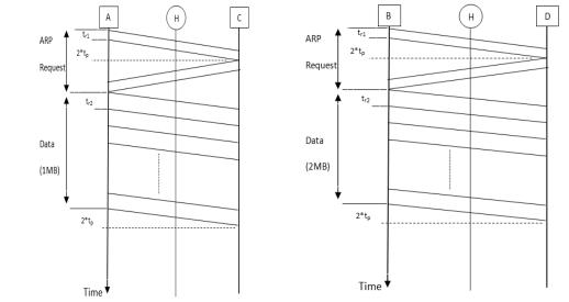
a) In the case of hub, the source will need first to make ARP request (packet size 64 Byte) to get physical address of destination so:
